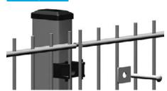
Post made of a 60x40x1.5 [mm] section, post h=3,200 [mm] 60x40x2 [mm]. Posts are supplied with a plastic cap and hooks for the panels with threaded holes for screws.
