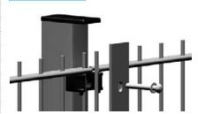
Post made of a 60x40x1.5 [mm] section, post h=3,200 [mm] 60x40x2 [mm]. The post is fitted with a plastic or aluminium (option) extended cap.
