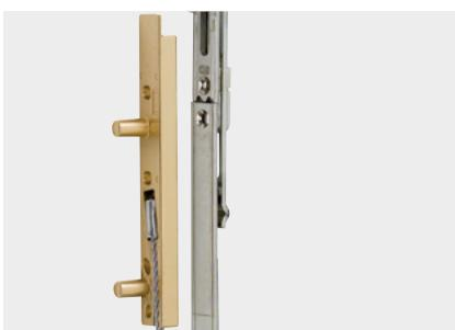
The Safety Pin secures each turn-only (side-hung) and turn and tilt window against leaf unhinging from the frame caused by mishandling. Located on the hinge side, the security device is integrated with the central turn and tilt locking system. The spring-loaded steel wire prevents the window leaf from falling out of the frame and effectively prevents potential accidents.
