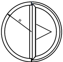
Minimum length of the welded sections of the frame/leaf for non-standard shape windows: 250 [mm]
