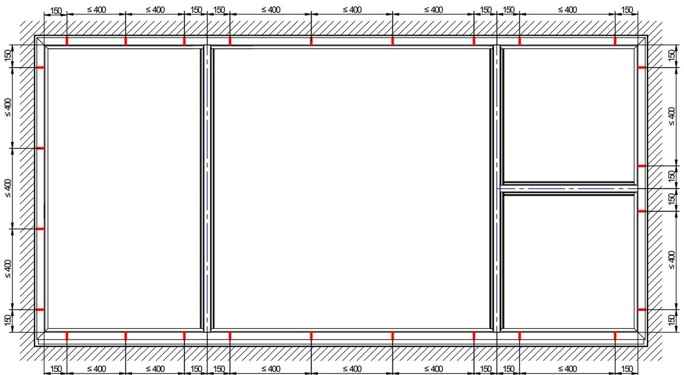
Marking for wall plugs is an option and is performed in accordance with the customer's requirements. Wall plug hole diameter –  $\varnothing 6$  [mm].
