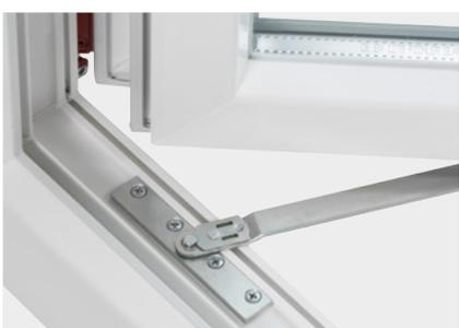
Fixes the opening angle of the leaf in the desired position. The brake stay can only be used in the R window version, but it cannot be used with a low threshold and with the RC and SECURITY enhanced burglary resistance class window versions.
