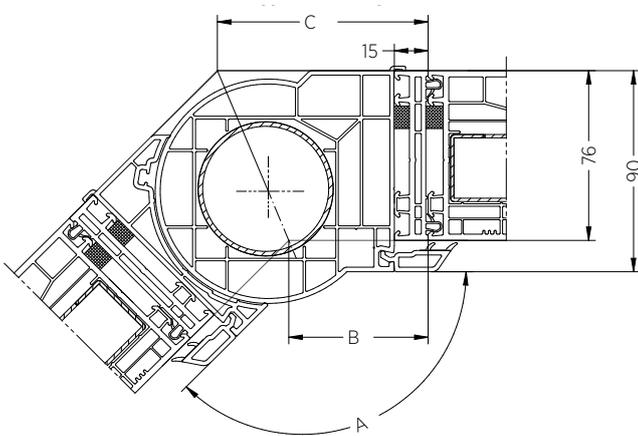
Pipe connector 116.216 + 114.052 with a 15 mm widening
