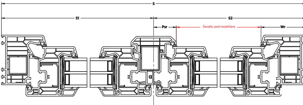
Clear opening for a mosquito screen, calculation formula:  $\text{Clear opening} = S2 - Wr - Psr$
