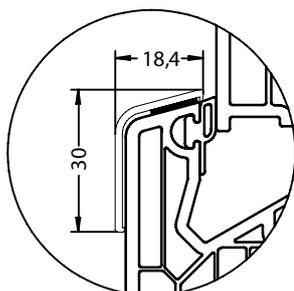
The aluminium threshold cover serves a protective function and prevents damage and scuffing of the lower part of the frame, it is especially recommended for balcony or patio exits.
