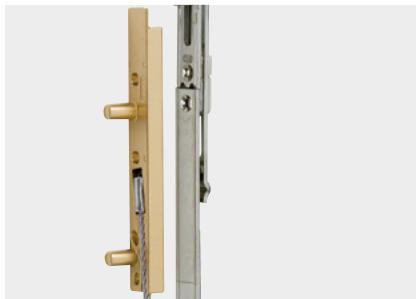
Safety Pin secures each turn-only (side-hung) and turn and tilt window against leaf unhinging from the frame caused by mishandling. Located on the hinge side, the security device is integrated with the central turn and tilt locking system. The spring-loaded steel wire prevents the window leaf from falling out of the frame and effectively prevents potential accidents.
